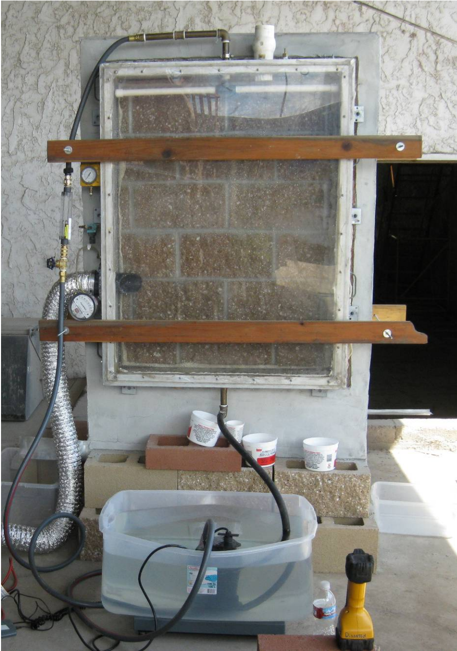
A single-wythe concrete block wall and ASTM E514 test setup. The clear box is pressurized to simulate wind, and the spray bar at the top of the box sprays water onto the block surface to simulate rain.
