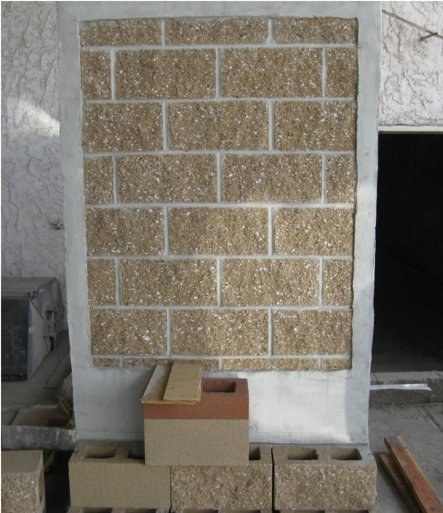
View of single-wythe concrete block wall prior to testing. The perimeter of the specimen is coated with plaster in accordance with ASTM E514 requirements.
